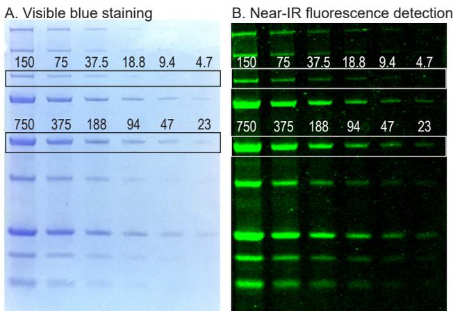
Figure 1. One-Step Blue®-stained SDS-PAGE gel. Two-fold dilutions of Unstained Precision Plus Protein™ Standard (Bio-Rad) were separated on a 1 mm thick Novex® NuPage® 4-12% Bis-Tris MES mini-gel (Thermo Fisher). The gel was stained with One-Step Blue® for 60 minutes. A) Visible blue staining. B) Near-infrared fluorescence in the 800 channel of a LI-COR® Odyssey®. Labels indicate approximate amount of protein (ng) in the boxed bands beneath.
